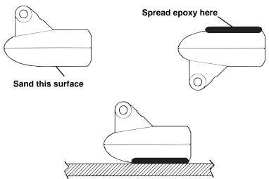
Epoxy transducer to hull.
